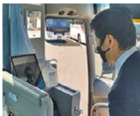
When it comes to fare payment, all a customer has to do is look at the facial recognition tablet without holding anything in their hands.
